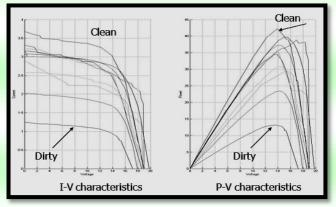
Figure 1 I-V and P-V characteristics of clean and dirty panels [1]
