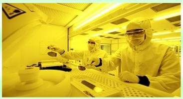
Figure 1 Dr Lai Nai Shyan performing resist coating in a class ten semi-conductor nano-fabrication clean room [4]
