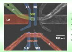
Figure 2 (Top view) Scanning electron microscope (SEM) image of a silicon quantum dot, with a charge sensor nearby.
